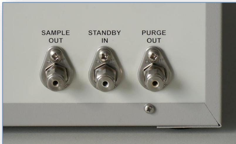
Referring to the diagram above connect the “Sample Out” to the analyser using 1/8 inch stainless steel pipe only. Ensure that all connections are tight, but **DO NOT** over tighten.
